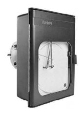
Barton Two Pen Pressure Temperature Recorder, Model 242E, Pressure Range: 0-5000 Psi, Mechanical Chart Drive: 24 HRs/7 Days
