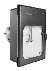
Barton Two Pen Pressure Temperature Recorder, Model 242E, Pressure Range: 0-5000 Psi, Mechanical Chart Drive: 2 HR/ 8 HR
