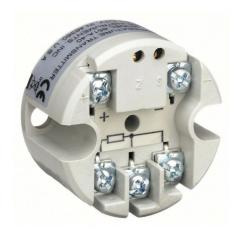
DWYER Temperature Transducer | Range 32 to 212 Degrees F | 10 to 32V DC, 651 | Type K Thermocouple, 4 to 20mA DC | Screw Terminals,
