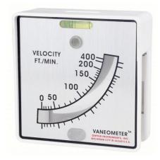
DWYER Anemometer | Range 25 to 400 fpm | Rotating Vane and Thermistor |  $\hat{A}\pm5\%$  Accuracy
