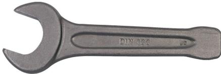
Forged and hardened steel. Flat striking faces to allow hammer blows to be used to loosen or tighten stubborn fasteners. To DIN 133.
