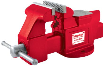
American pattern, bench mounting steel vice with anvil suitable for workshop, garage and machine-shop use. Fixed base directly mounts onto work bench. Cast iron body with steel jaws and a cross drilled threaded handle with adjustable T-bar for extra leverage.
