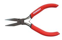
Made from high quality chrome nickel steel with induction ground cutting edges. Double dipped PVC grips for user comfort and control. Used for delicate, fine and accurate work in a continuous production environment. Spring loaded return for quick repetitive opening and operator comfort.
