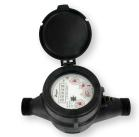
The Series WPT Multi-Jet Plastic Water Meter is a series of mechanical, water totalizing meters that display the total water usage in gallons with m<sup>3</sup> options. They are available in a range of body sizes and include NPT or BSPT optional couplings. The plastic body water meters can be used in potable water applications, some corrosive environments, or where an economical water totalizer is desired.
