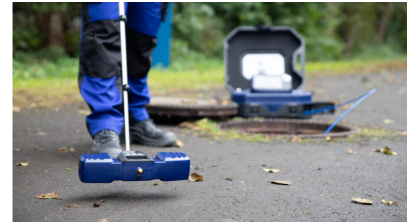
With the Wöhler L 200 Locator, the camera head can be located with pinpoint accuracy.
