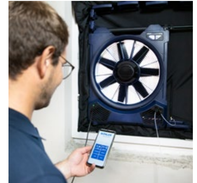
The fan unit is controlled via the Wöhler BC 600 app, which is simply downloaded to a smartphone, tablet or laptop (Android, iOS or Windows).
