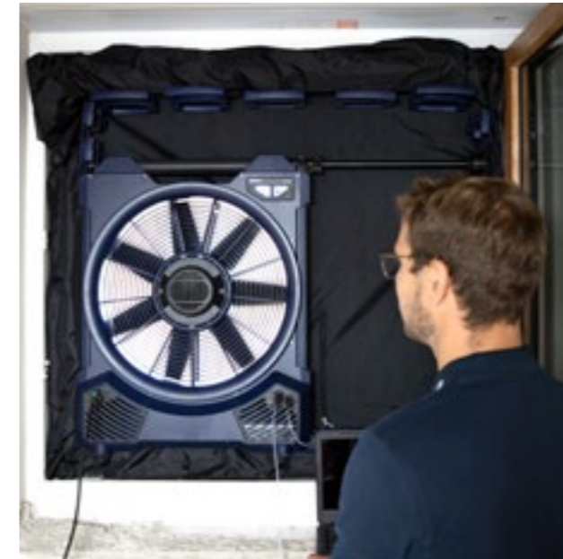
Fully automatic measurement sequence according to DIN EN ISO 9972 or DIN EN 13829 in the entire volume flow range from 15 – 6,000 m³/h without orifice plate change and overpressure and underpressure measurements without fan conversion.
