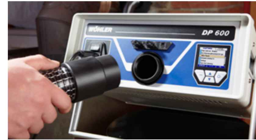
Setting up for measurement is easy: Just connect the pressure and air hose, input three values, and you're good to go!
