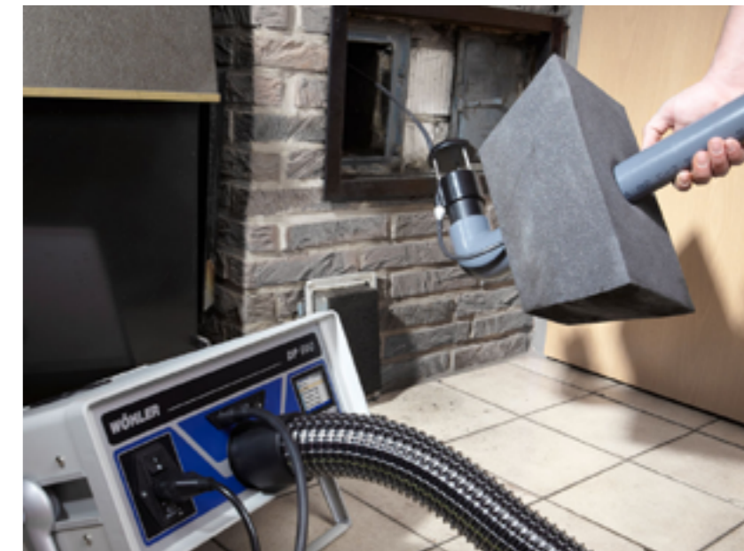
Ensuring safety and meeting standards: Testing a type N chimney under negative pressure conditions at either 20 Pa or 40 Pa.
