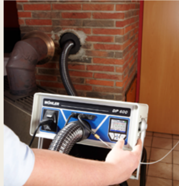
The 4 Pa Test can be carried out in a detailed procedure to prove that there is sufficient combustion air. The Wöhler DP 600 guides you safely through the measurement menu.
