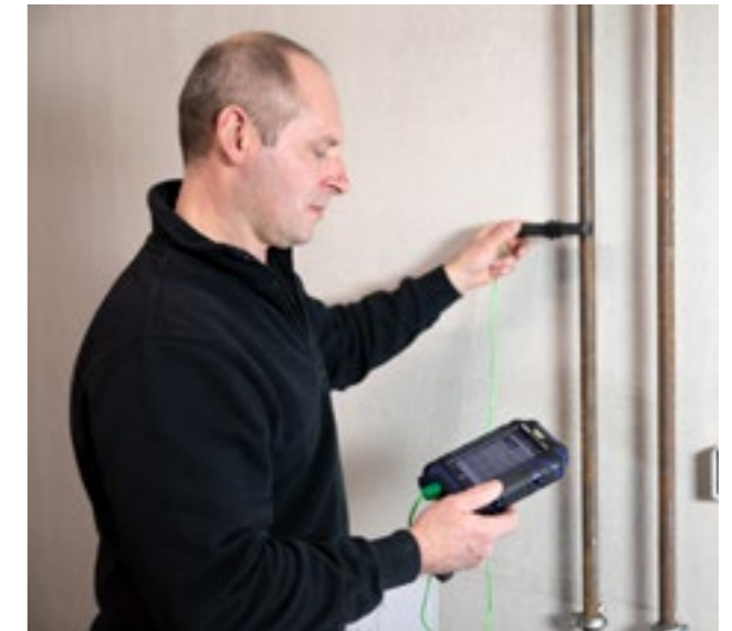
The temperature clamp probe can be used to determine the pipe temperature.
