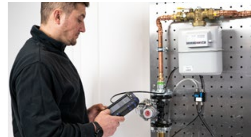
A separate menu item ensures that the functionality of the gas regulator can be tested in a few minutes.
