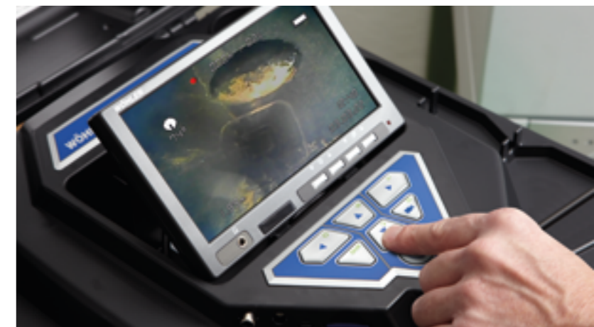
In addition to the digital meter counter, the display also shows the position of the head. The home button returns the camera head to its original position.
