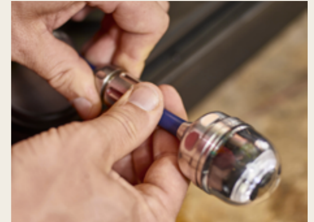
Thanks to the plugable Wöhler camera heads, pipes from Ø 40 mm to Ø 200 mm can be easily inspected. This picture shows the Wöhler pan & tilt camera head Ø 40.
