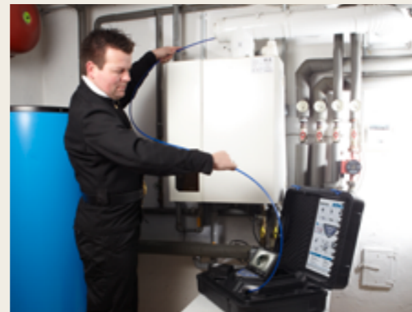
87° bends are effortlessly mastered by the colour camera head, which can be rotated 360° and swivelled 180°.
