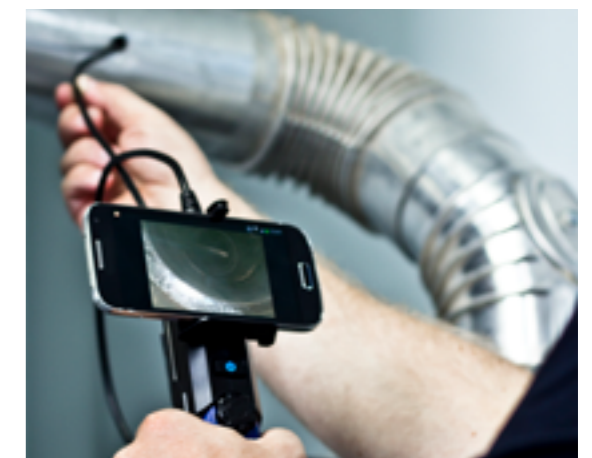
The images from the Wöhler VE 220 are also displayed in high quality on the smartphone. They can be conveniently sent from there.
