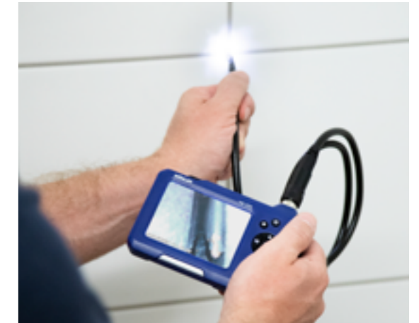
Just a Ø 4 mm opening in a tile cross is sufficient to inspect the installation behind the wall (Wöhler VE 320 in the picture).
