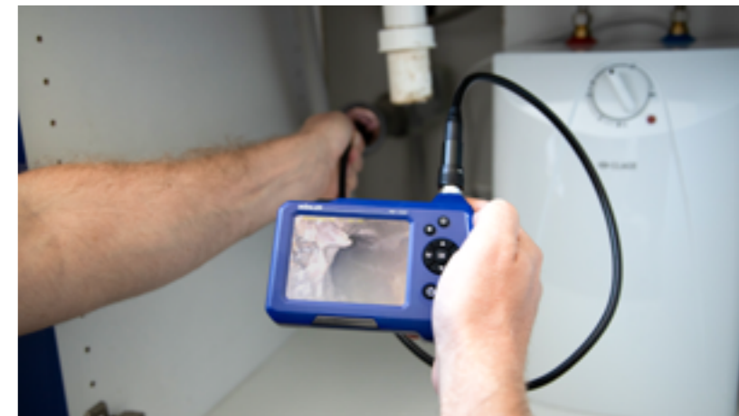
The display of the Wöhler VE 320 can be rotated by 180° for easy orientation in the pipe. The flexible probe manages bends with ease.
