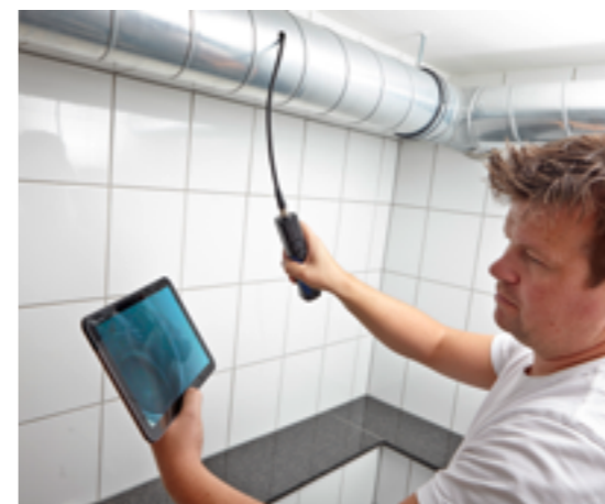
The small Wöhler VE 220 fits in every pocket. It transmits the image and video files via Wi-Fi to your mobile device and if desired also simultaneously to your tablet and smartphone.
