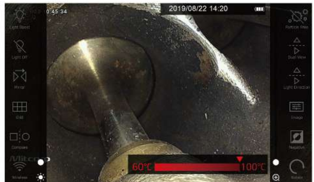
3 stage temperature warning & auto shut down function
