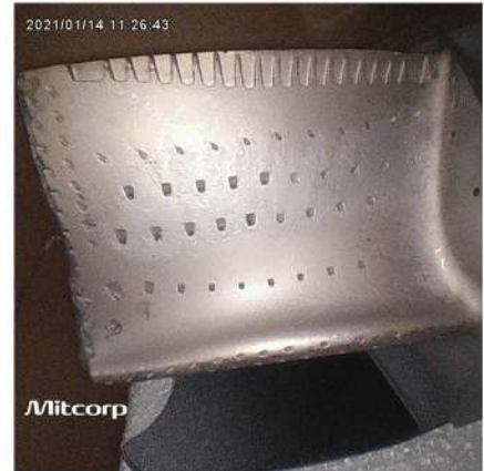
1600*1600 output by 3.9mm HD probe (30mm distance)
