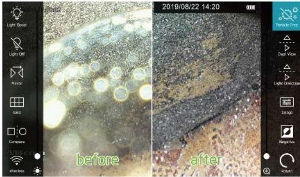
Patented particle free effect (with mirror)
